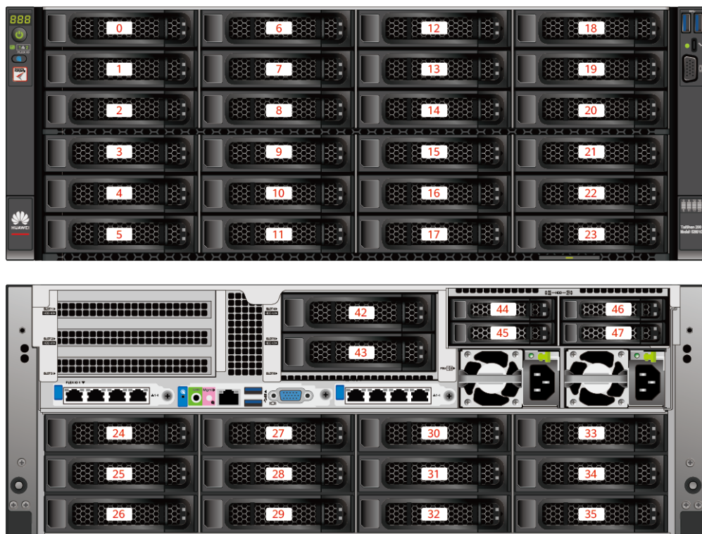
Figure 5-9 Drive numbers of a server equipped with 36 x 3.5-inch SAS/SATA drives
